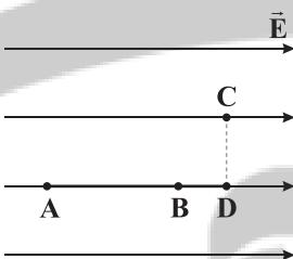
$$E_A = E_B = E_C = E_D, V_A > V_B > V_D > V_C \quad (1)$$
