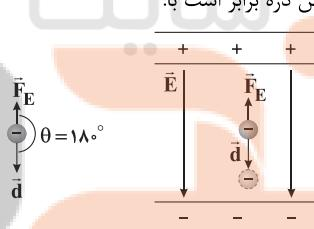
$$W_E = F_E d \cos \theta \xrightarrow{\theta = 180^\circ} W_E = F_E d \times (-1) \Rightarrow W_E = -F_E d$$
