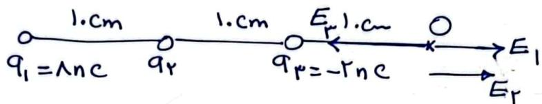
$$E_1 = k \frac{q_1}{r_1^2} = q \times 1.0 \times \frac{1 \times 10^{-9}}{q \times 1.0^2} = 1 \mu N/C \rightarrow \vec{E}_1 = 1 \mu \text{N} \vec{i}$$
