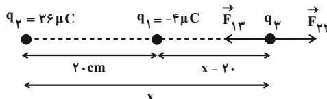
$$F_{13} = F_{23} \Rightarrow k \frac{|q_1||q_3|}{r_{13}^2} = k \frac{|q_2||q_3|}{r_{23}^2}$$
