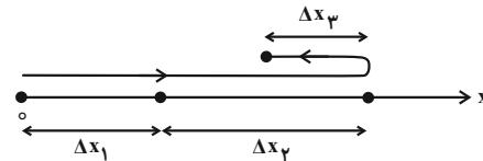
$$v_{av} = \frac{\Delta x_3}{\Delta t_1 + \Delta t_2 + \Delta t_3} \quad \Delta x = v_{av} \Delta t$$
